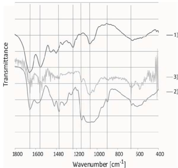
Fig. 1. FTIR spectra of homogeneous Coll film (1), MCCh film (2) and MCCh-Coll composite membrane (2:1) (3)
