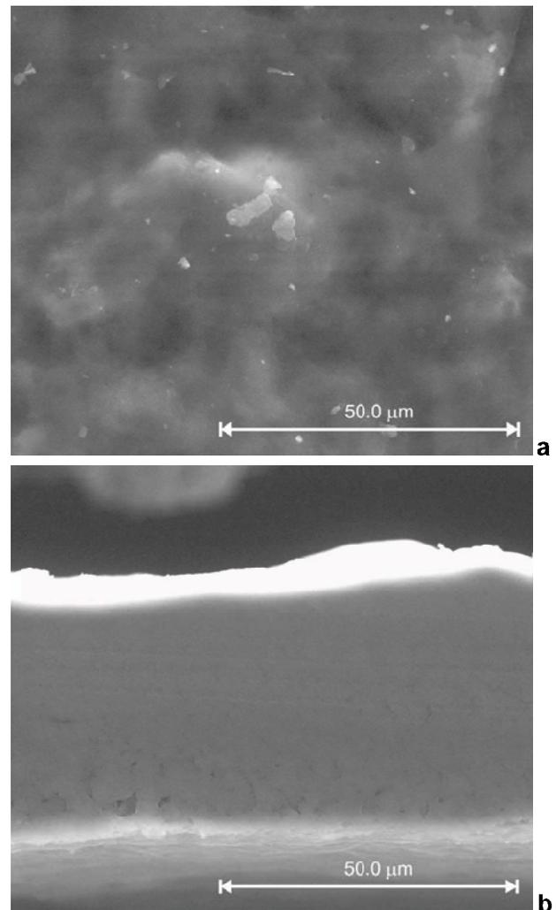
Fig. 3. SEM image of microcrystalline chitosan-collagen (MCCh-Coll) composite membrane a) membrane surface, b) cross-section –  $\times 3000$
