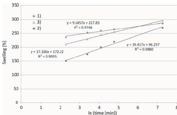
Fig. 2. Swelling percentage of 1) ♦ MCCh, 2) ■ Coll and 3) ▲ MCCh-Coll membranes in distilled water after 10, 30, 60, 120 and 1440 min. Values are average of six determinations
