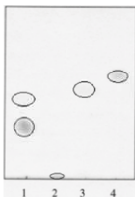
Fig. 1. TLC chromatogram of fraction of triterpenoids from Scirpus maritimus L. and Carex paradoxa Willd. in comparison with standards of lupeol and \beta -amyrine in a system : chloroform : diethyl ether(19:1) (1 – Fraction of triterpenoids from Scirpus maritimus L.; 2 – Fraction of triterpenoids from Carex paradoxa Willd.; 3 – lupeol; 4 – \beta -amyrine)
