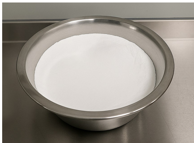
Figure 5. Formulation F2 after high-shear mixing (dry-coating)
