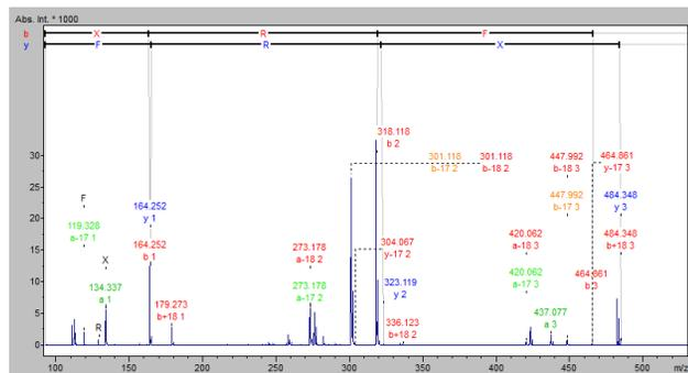
**Figure 4.** MS/MS MALDI-TOF mass spectrum of a protonated molecule of RF9 (m/z 483.3) confirming its presence after the synthesis. Data shown for COMU/DIPEA method. X on the mass spectrum stands for 1-adamantanecarboxylic acid residue
