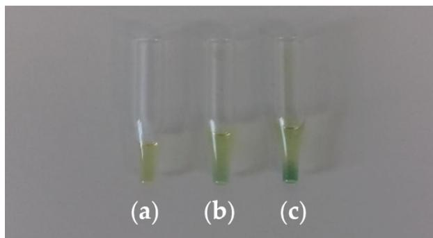
**Figure 1.** Chloranil test after 1-adamantanecarboxylic acid substitution with carboxylic acid activation by: (a) COMU/DIPEA, (b) DIC/HOBt and (c) only DIC
