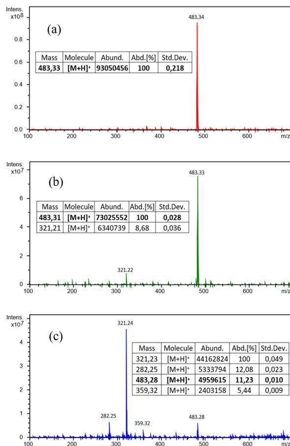
**Figure 2.** ESI mass spectra obtained for the RF9 synthesis after different carboxylic acid activation methods at the last stage of the synthesis: (a) COMU/DIPEA, (b) DIC/HOBt and (c) only DIC. Inserted tables contain information higher than 5% of relative abundance. The peak corresponding to a desired product is bolded in the tables
