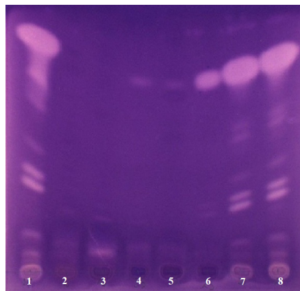
Figure 1. Videoscans of TLC with bioautography – the application of the modified 'Fast Blue B reagent' method. Here, the presence of potent AChE inhibitors is indicated by white inhibition zones on a deep purple background. The tracks follow fractions obtained from Narcissus triandrus L. c.v. 'Hawera' using PLE and VLC
