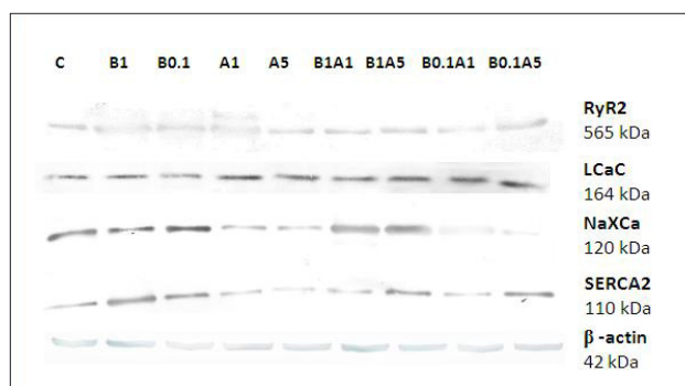
Figure 4. Representative Western blot analysis for RyR2, LCaC, NaXCa, SERCA2 proteins in the rat cardiomyocyte H9C2 line. Beta-actin is shown as a loading control
